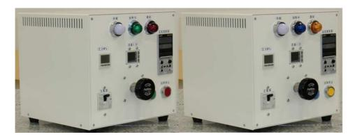
By overheating zero setting of the thermocontroller, it makes the stable hot-air heating. At a flow rate management by the flow control valve with a float-type flow meter or mass flow controller, to ensure the reproducibility of the amount of heat supplied.
